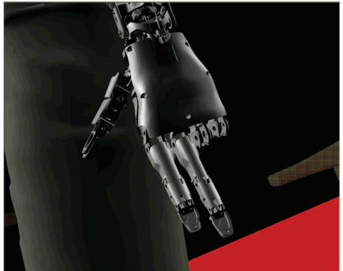
Fig. 4. Screenshot of the VIE's virtual prostheses as individual finger movements are being decoded (middle finger extension depicted). The data was collected from EMG from a transradial amputee, then streamed and decoded in real-time.
